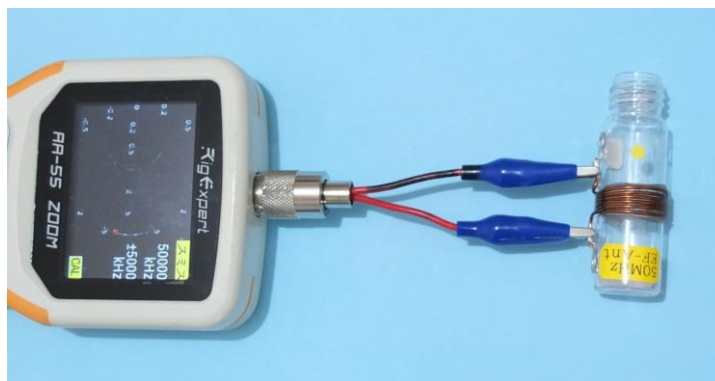
Photo2.1 Inductance measurement status
